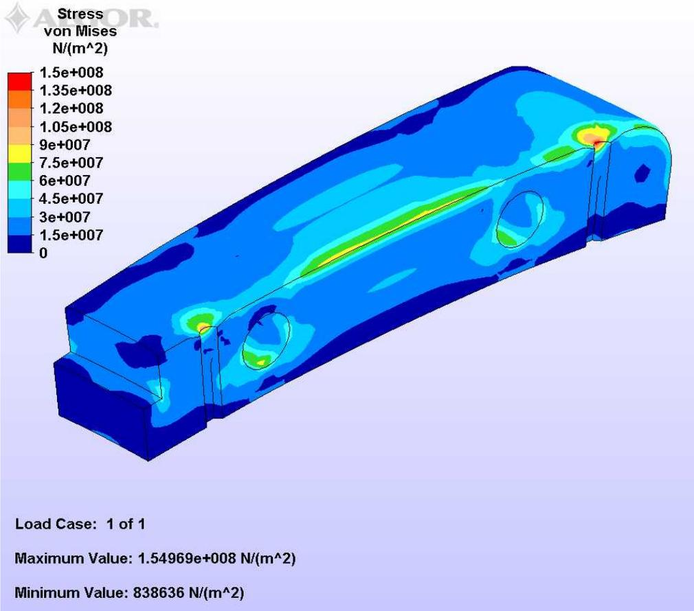
*Mechanical stress significantly reduced well below the TZM allowable (<400 MPa) when moly tile is allowed to bow upwards ( $P_{Av} = 1MW/m^2$  for 2 second)*
