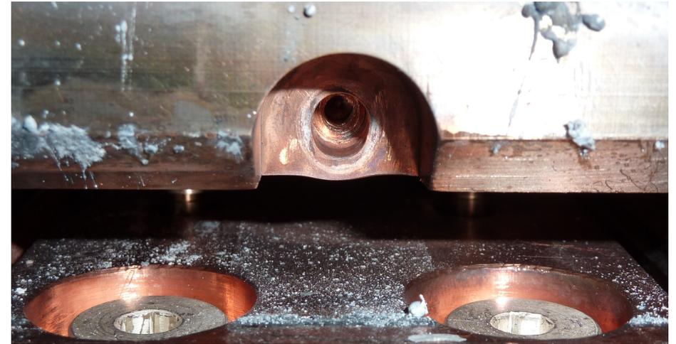
Arc damage in LLD heating tubes and Center Post
