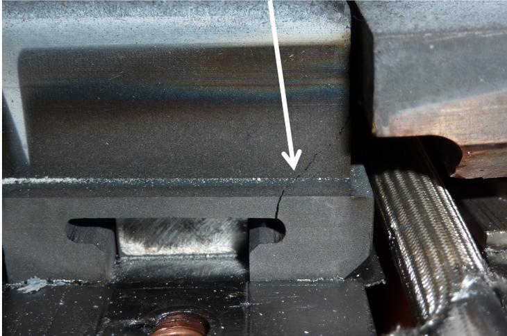
LLD support hole elongated due to excessive stress
