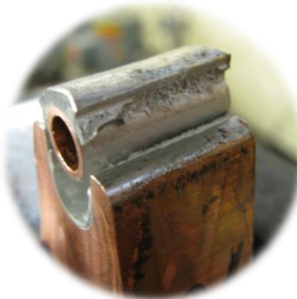
Solder paste injection over cooling tube
