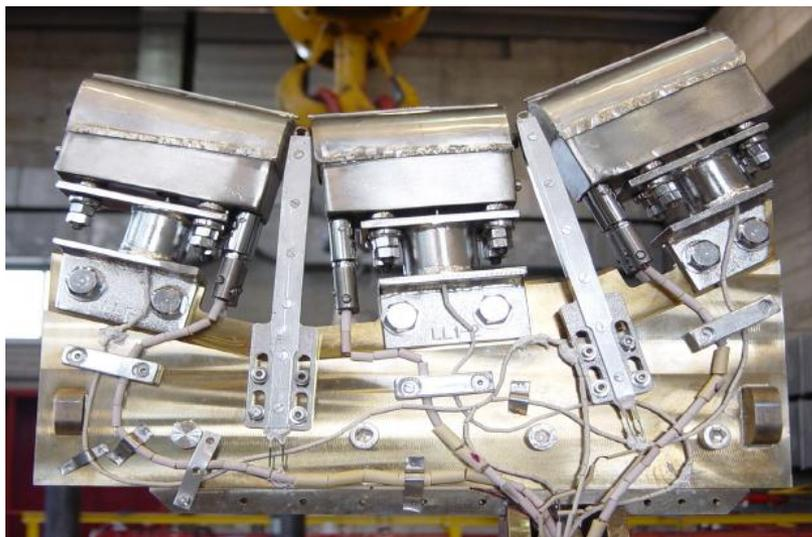
FTU capillary porous system (CPS)
