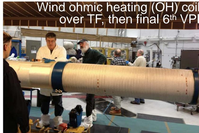
Wind ohmic heating (OH) coil over TF, then final 6<sup>th</sup> VPI
