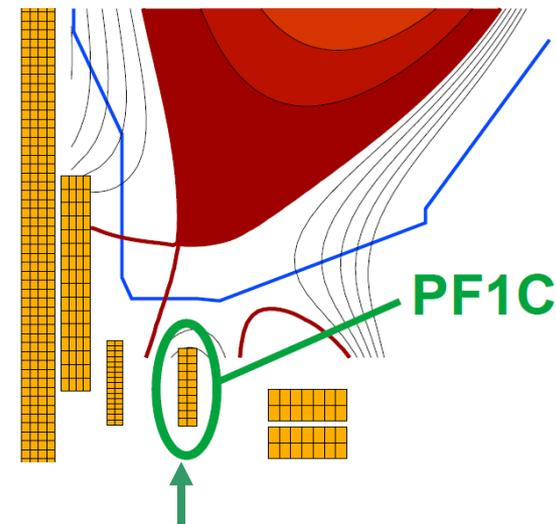
**NSTX-U has additional coils for up-down symmetric snowflake/X, improved control**
