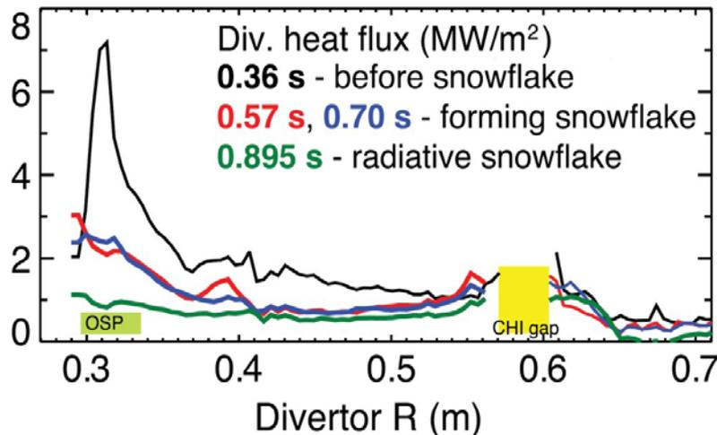
**NSTX-U peak heat fluxes will be up to  $4-8 \times$  higher than in NSTX**
