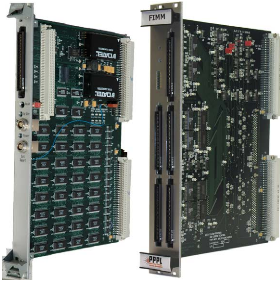
Fig. 2. Shown on the left, the Stand-Alone Digitizer (SAD) developed at PPPL, is a simple 32 channel FPDP digitizer. Shown on the right is the Front Panel Data Port Input Multiplexing Module (FIMM) developed at PPPL combines multiple FPDP streams.
