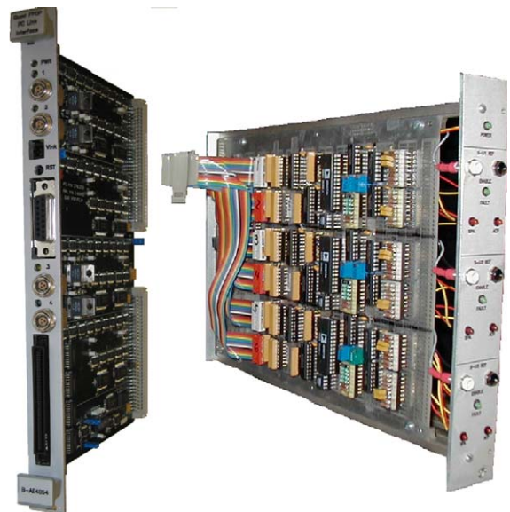
Fig. 3. The PCLIM module (left) interfaces the FPDP output stream with the legacy PCLink interface that was inherited from TFTR while the SPAIM (right) interfaces FPDP to a switching power amplifier with analog inputs.
