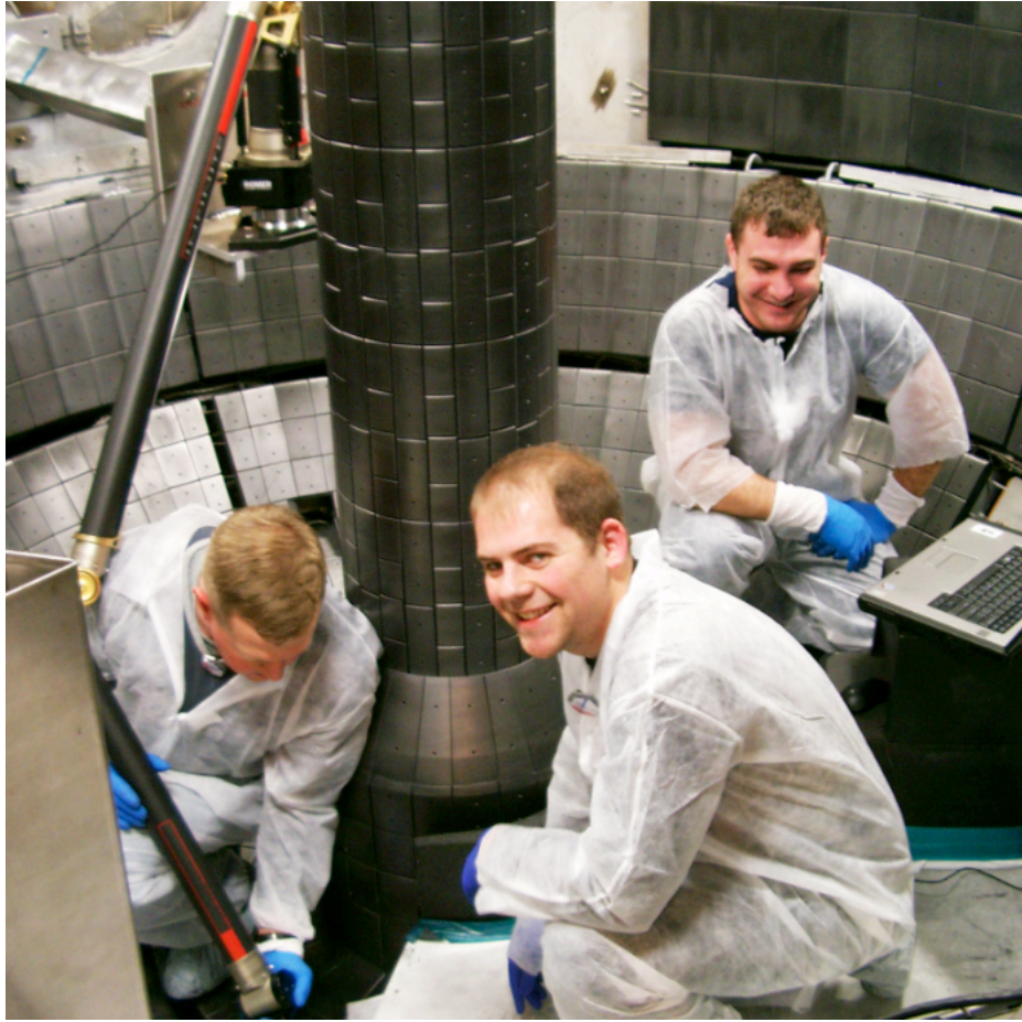
Figure 4.23: The author along with Craig Priniski and Dan Stevens measuring the probe locations in NSTX
