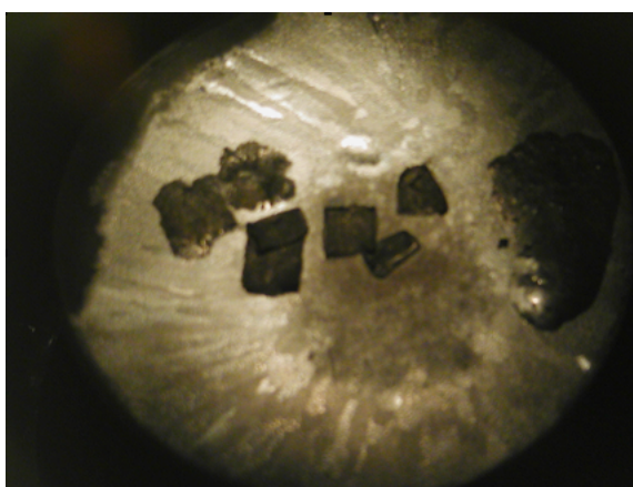
Figure 3.19: Li substrate following reheating and cold glow tests
