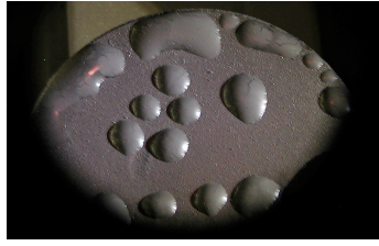
Figure 3.13: Passivated sample after LITER evaporation
