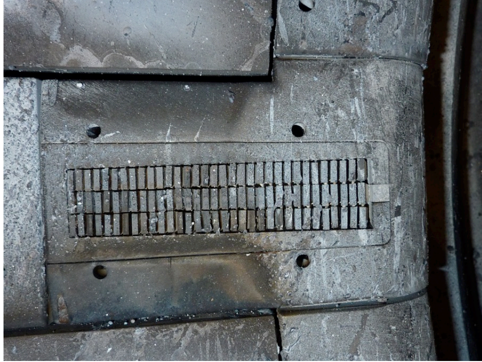
Figure 4.24: Probe array after 2010 run year, pre-cleaning
