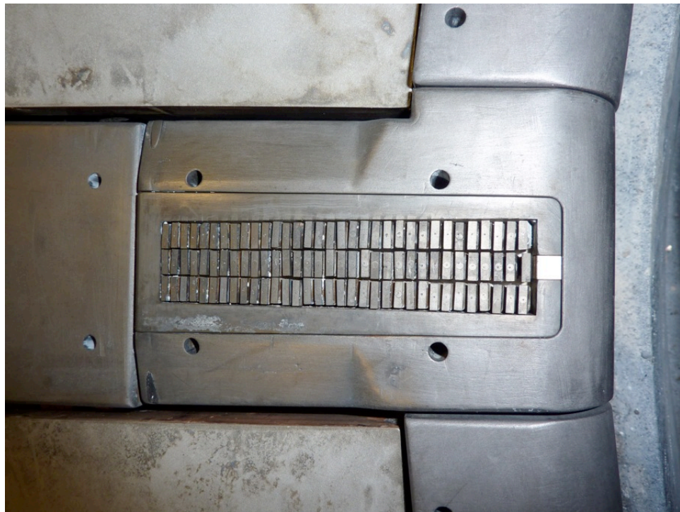
Figure 4.25: Probe array post-cleaning
