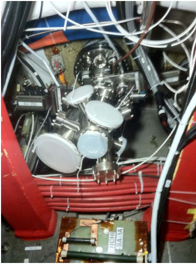
Fig. 2. Picture of MAPP analysis system attached to NSTX TIV, illustrating the tight space constraints for all equipment.
