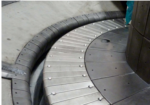
Fig. 5. Photograph showing row of TZM PFC tiles on IBD bottom divertor in NSTX. Gap for CHI can be seen to the left of the tiles.
