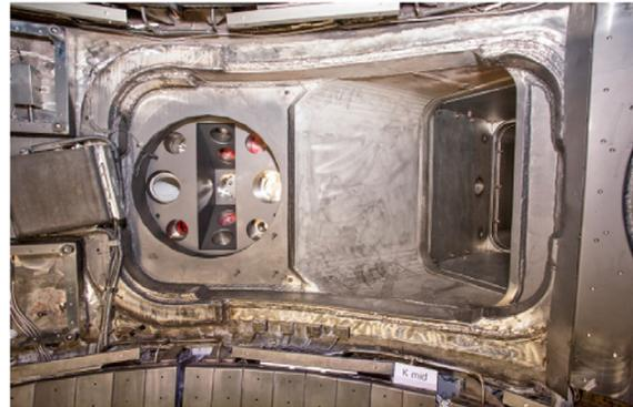
**Figure 15.** In-vessel view of the tangential injection port of the 2nd NBI.
