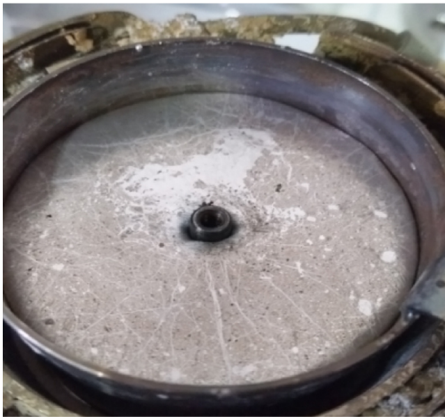
Fig. 4. The surface of \text{Ga}_{67}\text{In}_{20.5}\text{Sn}_{12.5} after plasma exposure experiments, showing a buoying contamination film.
