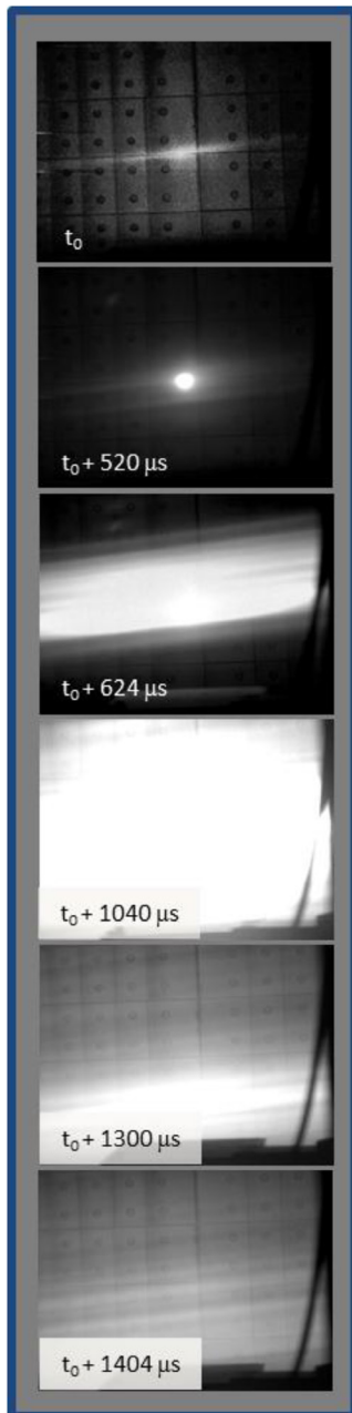
Figure 5. Selected frames captured during injection of an \sim 700 micron lithium granule displays the stages of the ablation event. Frame 1 brightened to show detail.
