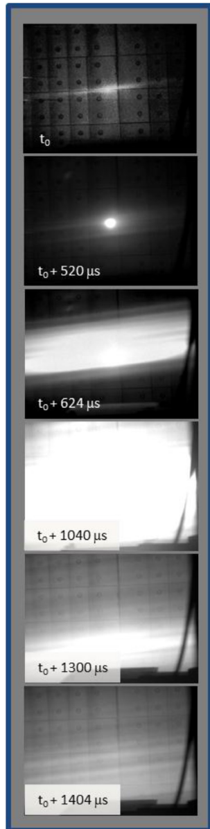
Figure 5. Selected frames captured during injection of an \sim 700 micron lithium granule displays the stages of the ablation event. Frame 1 brightened to show detail.
