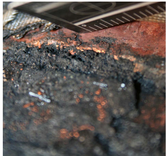
Fig. 18. Layer 2 conductor No. 30 electrical activity.
