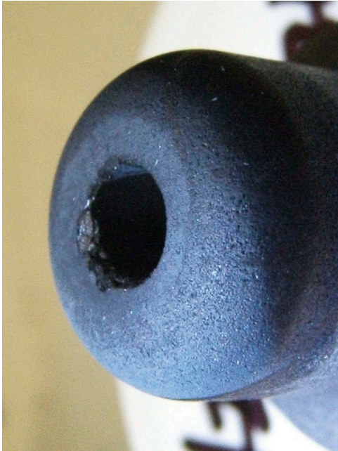
Fig. 15. Photograph of SGI nozzle eroded by plasma after 6 years of operation.
