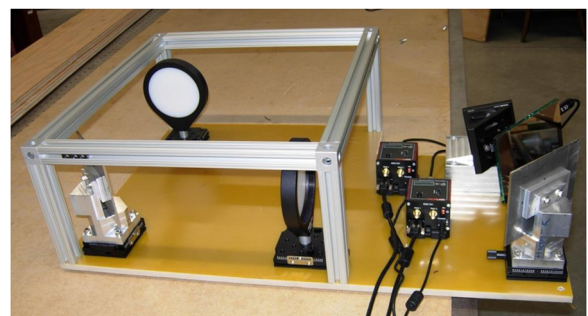
FIG. 7. Photograph of the high- k_0 launch optics assembly, mounted on a G11 backboard, with Lexan paneling removed.
