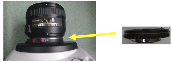
FIG. 4. The filter is inserted in-between a Nikon lens and the camera sensor, when in use.
