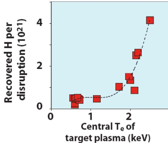
Fig. 12 Hydrogenic fuel recovery on C-Mod following intentional disruptions with varying target plasma  $T_e$  (at constant density). [2]
