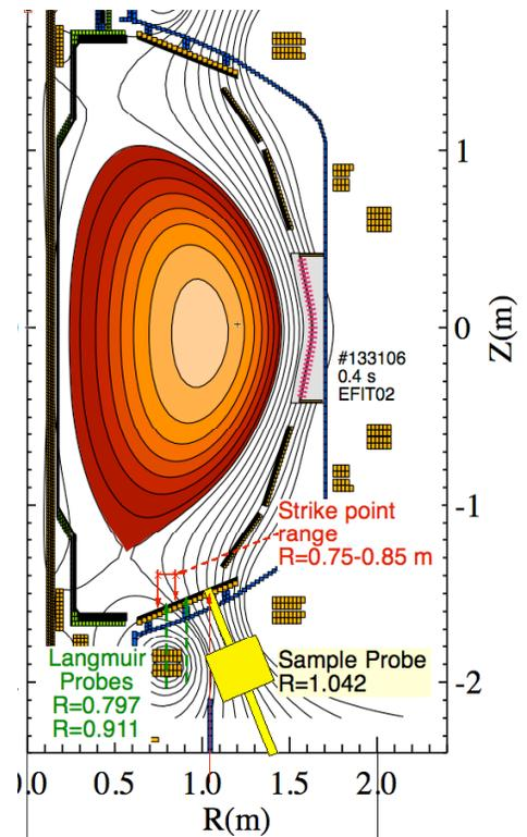
Fig. 2 Discharge magnetic geometry with sample probe location.
