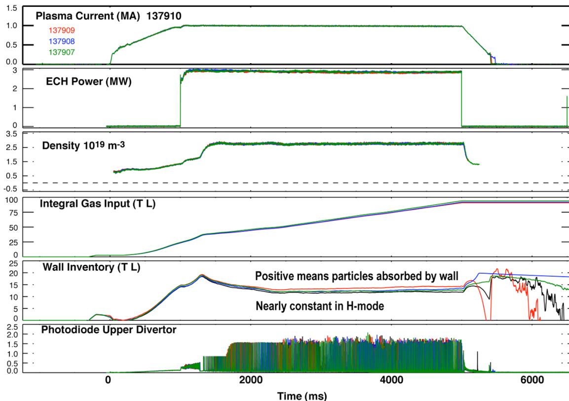
Fig. 14. The plasma current, electron density, gas fueling rate, and ECH power is shown for a series of four reproducible ECH H-mode DIII-D shots. The results from the dynamic particle balance for the wall inventory are shown; the sign convention on the wall inventory is that a positive value means that wall is removing particles from the plasma. Note that the wall inventory increases during the startup and L-mode period of the plasma, but during H-mode, the wall flux is very small.
