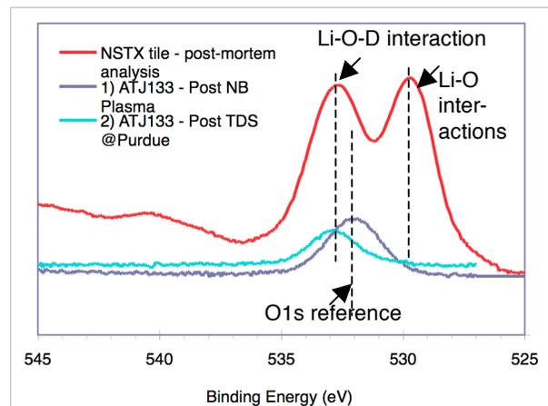
Fig. 6 Oxygen 1s spectrum of X-ray photoelectron spectroscopy (XPS) at Purdue Univ. of ATJ graphite sample exposed to 6 NSTX neutral beam heated lithium conditioned plasmas.
