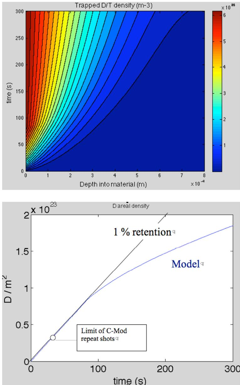
Fig. 9 Numerical simulation of D retention in Mo at divertor with surface trap production and mobile traps. (Top) Contour of trapped D versus time and depth into Mo (Bottom) Integrated D fluence retained.
