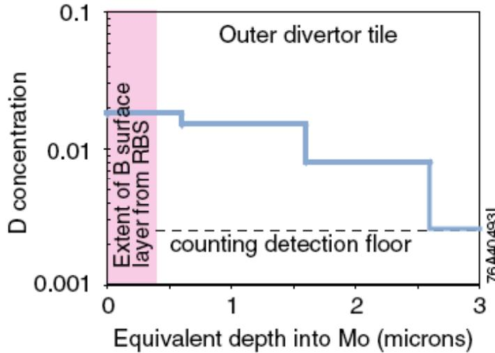
Fig. 8 Post-campaign Deuterium depth profile in Molybdenum tile using Nuclear Reaction Analysis. D concentration is normalized to Mo atom density [1].
