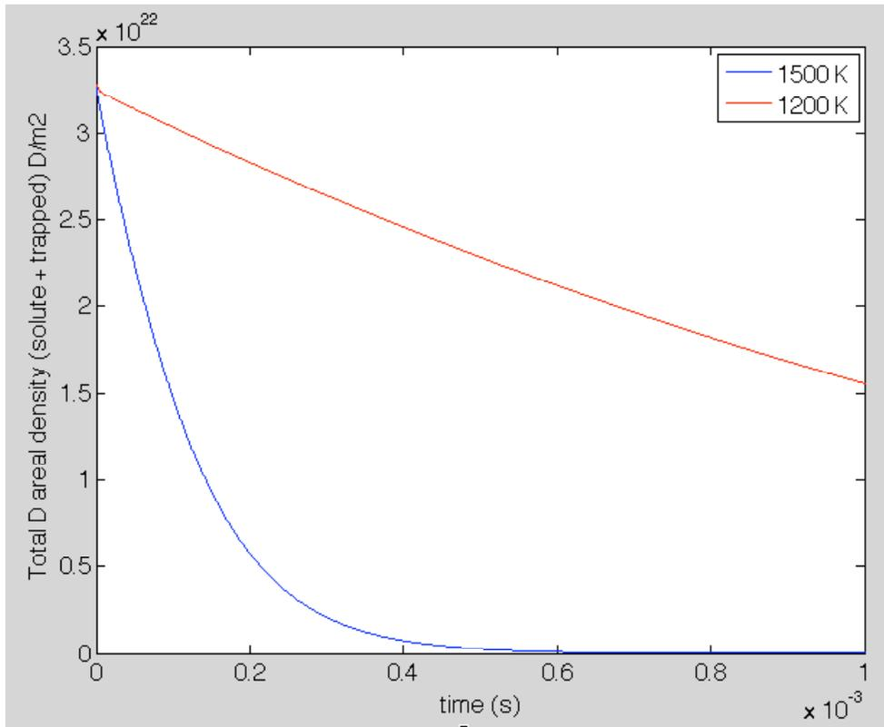
Fig. 13 Simulation of disruption-heating induced reduction of retained D in Mo for two different assumptions of surface temperature.
