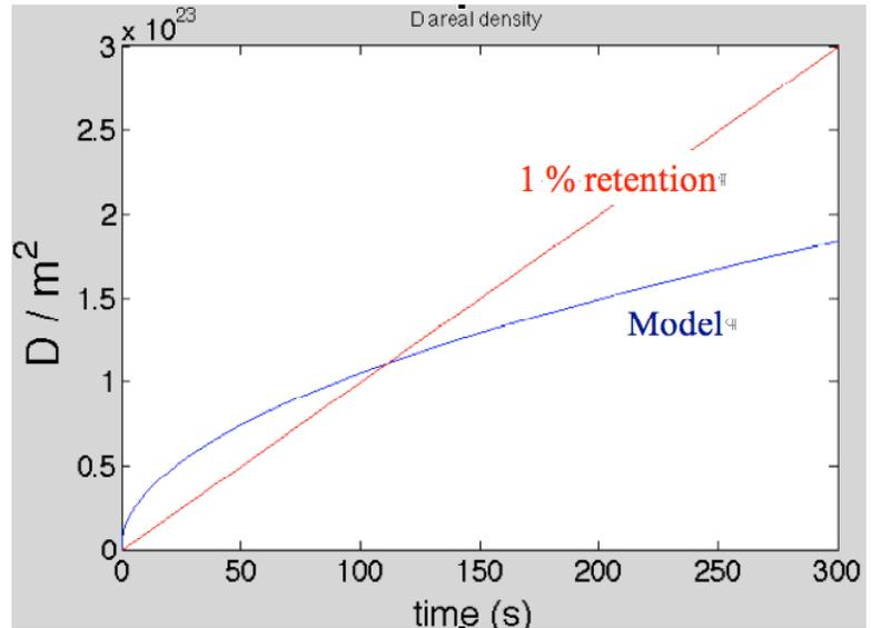
Fig. 10 Numerical simulation of D retention in Mo at divertor with immobile traps at 1% concentration.
