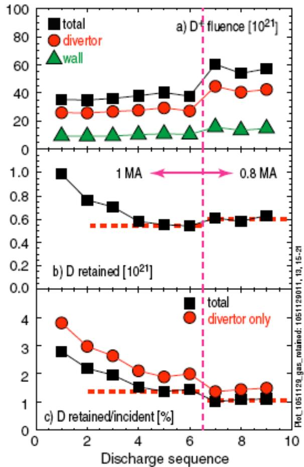
Fig. 7 Deuterium fuel retention on C-Mod in a sequence of repeated discharges. [1]
