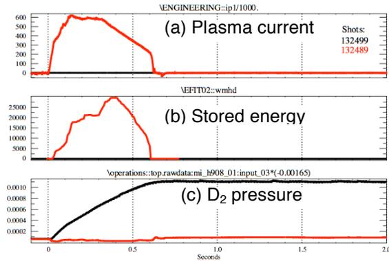
Fig. 3 (a) plasma current (b) stored energy (c) deuterium pressure for ohmic and gas-only pulses before Li conditioning. The prompt retention is 93%.
