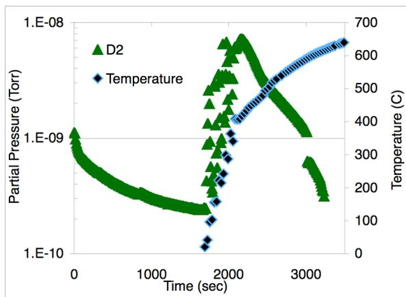
Fig. 5 Same-evening thermal desorption spectroscopy of ATJ graphite sample exposed to 6 NSTX neutral beam heated plasmas.
