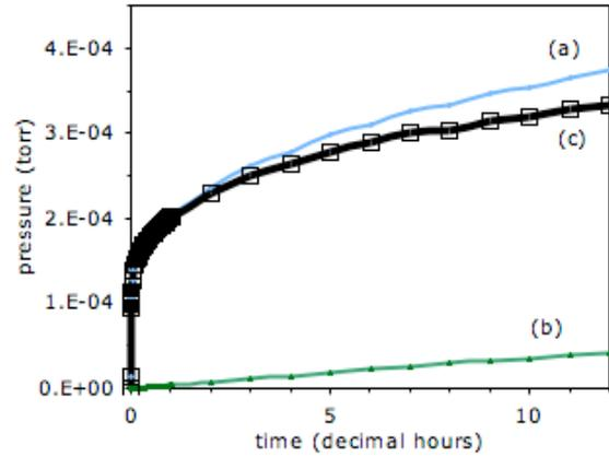
Fig. 4 Pressure rise over 12 hours (a) deuterium (b) nitrogen leak rate (c) difference .
