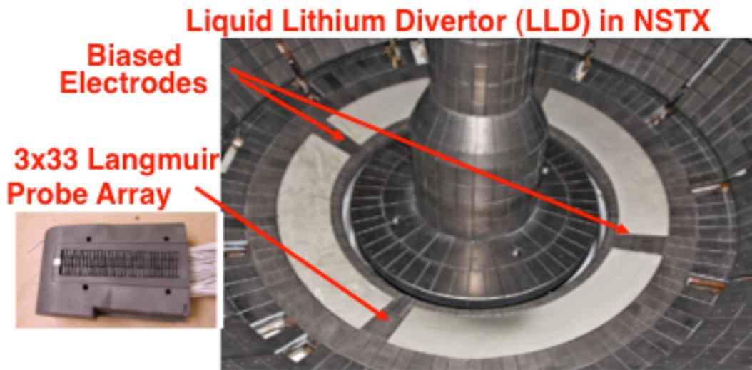
*Figure 7 – NSTX Liquid Lithium Divertor (LLD) target plates installed in NSTX.*
