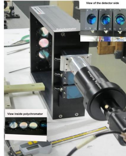
**Additional 12 channels enhance resolution in pedestal to ~1 cm and improve diagnosis of ITB in plasma core**
