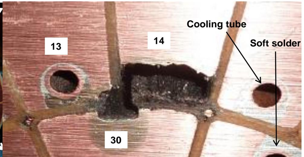
**TF Upgrade will use rosin flux and change the procedures for removing the flux residues**
