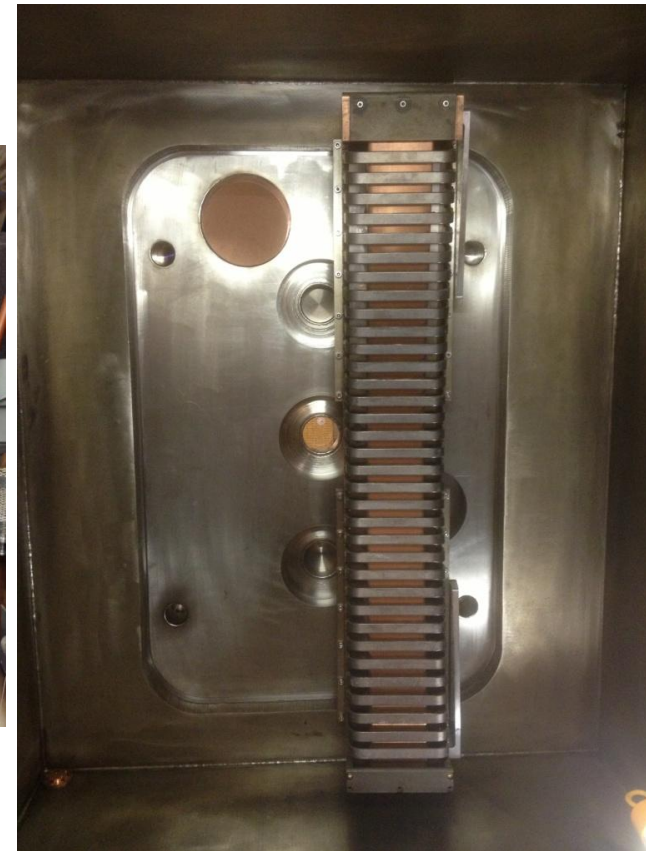
Inside of RF Test Stand with one antenna assembly.
