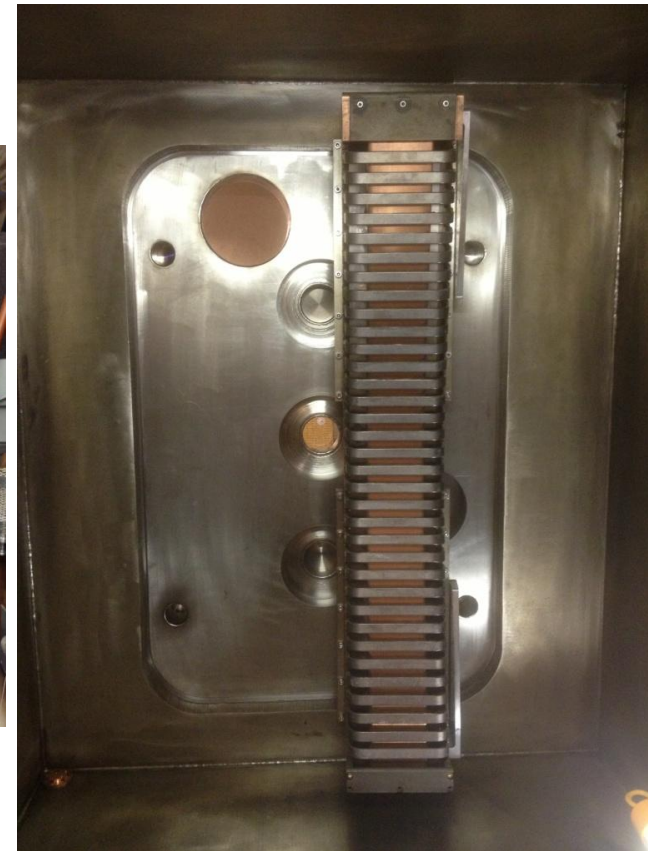
Inside of RF Test Stand with one antenna assembly.
