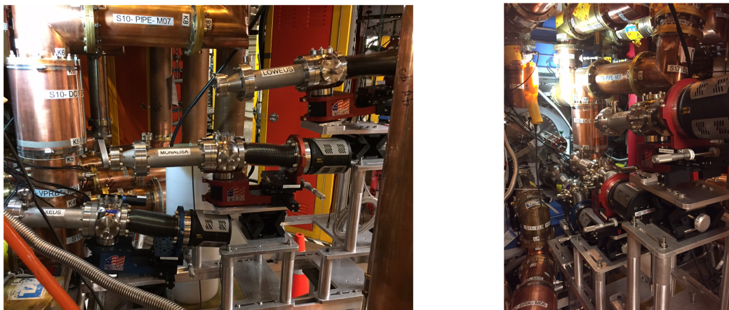
Figure FD-17: New mounting system for the three EUV spectrometers XEUS, MonaLisa, and LoWEUS.
