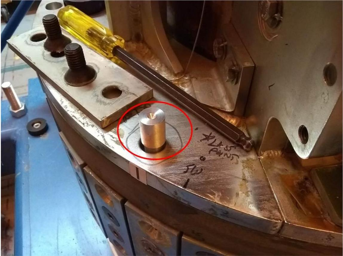
**Fig. MET-7:** Custom threaded gauge made to measure Keensert locations in bottom support (E-DC1482).
