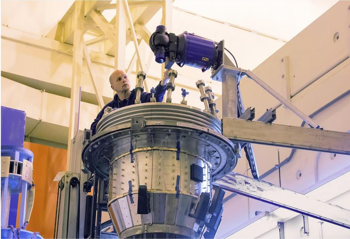
**Fig. MET-3:** Machine Tech Scott Gifford with horizontally-mounted laser tracker atop CS Casing.
