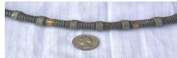
Diamond wire used to section torus
