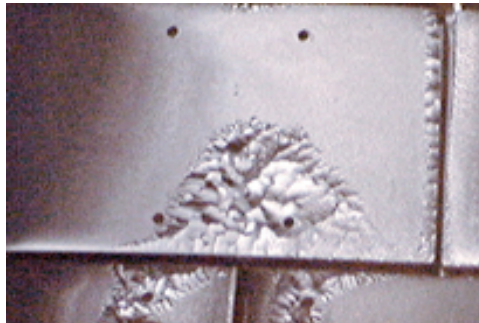
Flakes from tile KA7. (plasma facing, inner limiter)
