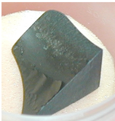
Flakes from diagnostic penetration on tile KC22 (not plasma facing)
