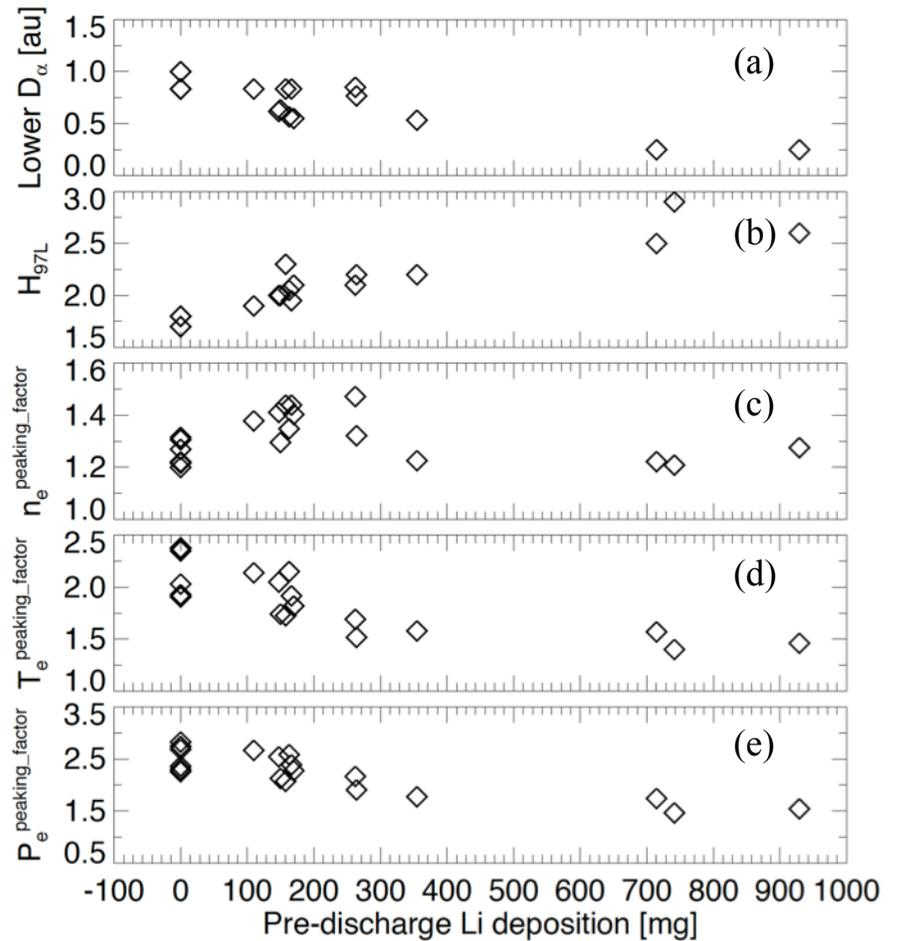
Figure 1: Evolution of plasma parameters as a function of pre-discharge lithium ‘dose’: (a) Lower divertor  $D_\alpha$  baseline value at  $t=0.4$  sec, (b) energy confinement relative to ITER97-L scaling, (c)  $n_e$  profile peaking factor, (d)  $T_e$  profile peaking factor, and (e)  $P_e$  profile peaking factor. Panels (b)-(e) were computed at the time of peak  $W_{MHD}$ . [Maingi, PRL 2011 submitted]
