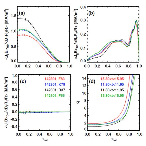
AII:  $E_{inj}$ =90 kV,  $P_{inj}$ =8.4 MW,  $B_{T}$ =1.0 T,  $H_{98y,2}$ =1,  $f_{GW}$ =0.7,  $f_{Ni}$ =100%  $R_{tan}$ =[50,60, 70, 130] cm,  $I_{p}$ =675 kA,  $q_{min}$ =1.88  $R_{tan}$ =[50,60, 120,130] cm,  $I_{p}$ =740 kA,  $q_{min}$ =1.54  $R_{tan}$ =[60,70, 110,120] cm,  $I_{p}$ =770 kA,  $q_{min}$ =1.03  $R_{tan}$ =[70,110,120,130] cm,  $I_{p}$ =800 kA,  $q_{min}$ =1.51
