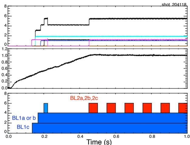
Fig. 1. a) Beam waveforms for shot 204118, b) plasma current waveform, c) proposed beam waveform.
