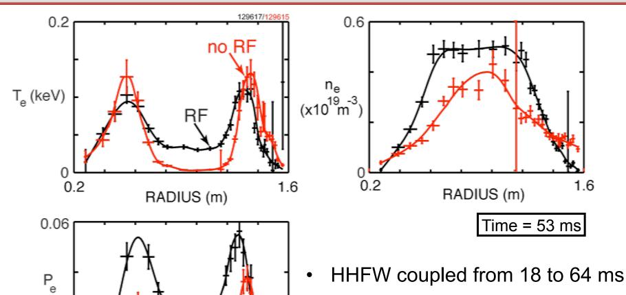
T<sub>e</sub>, P<sub>e</sub> profiles remained hollow during HHFW heating pulse
