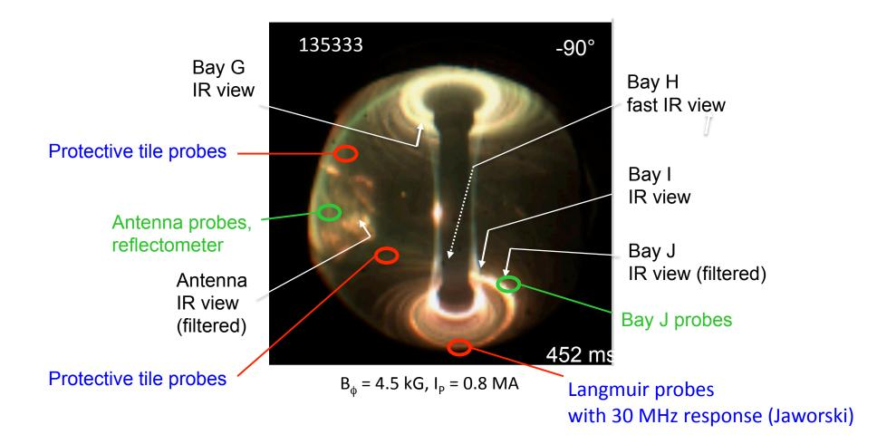
Need probes in protective tiles under and above antenna and in same vertical locations away from field lines that pass in front of the antenna
