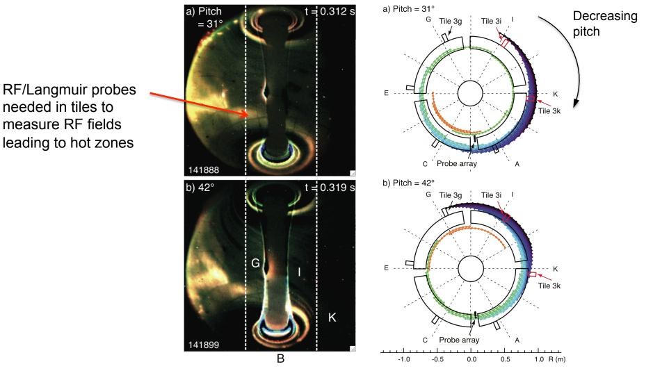
Reduced magnetic pitch will allow direct comparison between fast wave results on NSTX and DIII-D
