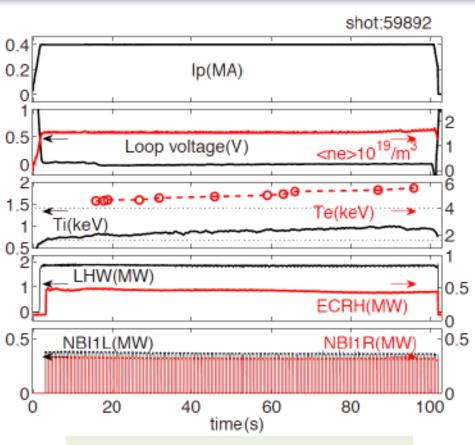
100s high electron temperature (Te > 4.5keV) operation
