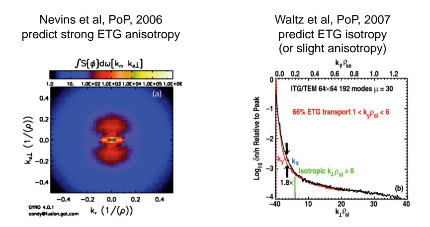
ETG radial streamers are anisotropic features (simulations above do not use the same plasma conditions)
