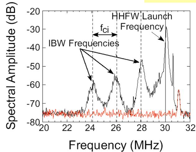
Evidence for parametric absorption processes found in spectroscopy, RF probes
