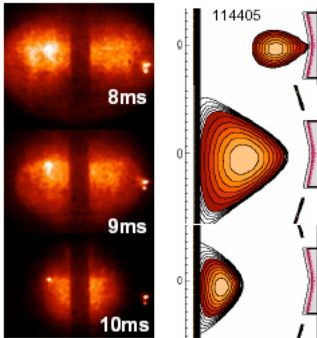
Need to maintain plasma on outside where  $V_{loop}$  is high
