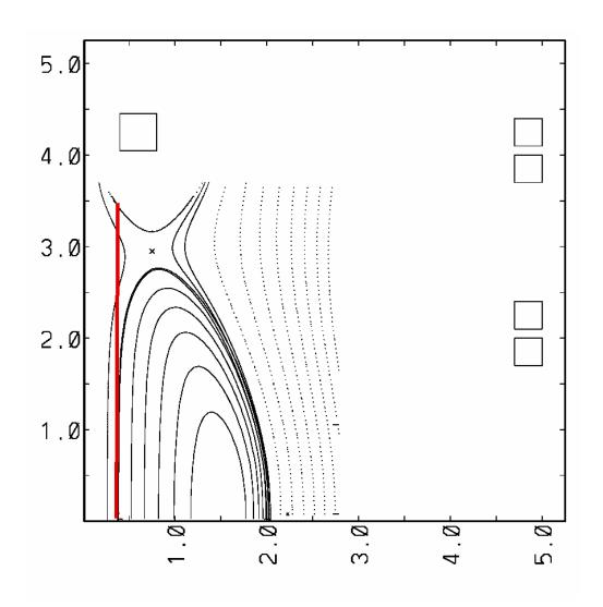
Both Inboard Limited & Double Null Diverted Plasmas Can be Produced as Long as Low  $\ell_i$  is maintained
