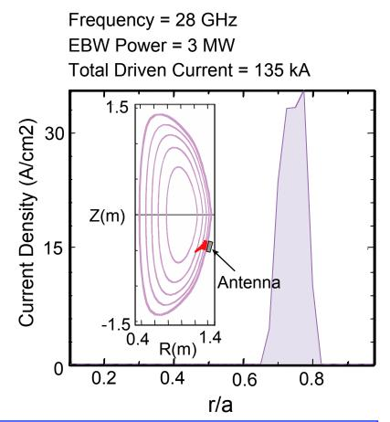
EBW ray tracing, deposition and CD efficiency being studied with GENRAY & CQL3D for frequencies between 14 to 28 GHz
