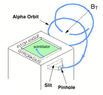
Scintillator detector: principle of operation
