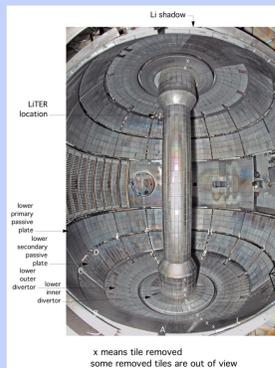
PPPL removed 23 Si witness samples (ws) from NSTX. After the samples were exposed to atmospheric conditions, a passive oxidized layer began to form on the surface. In addition, three tiles were cored yielding about 5 samples per tile. Analysis of these samples at Purdue University indicated the need of conducting control experiments with *in-situ* analysis to avoid ambient air exposure effects. These control experiments will provide complementary data to post-exposure analysis at Purdue.
