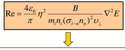
If  $\nabla^2 E \sim 0$ , Re can be smaller than Re\* which determine turbulence
