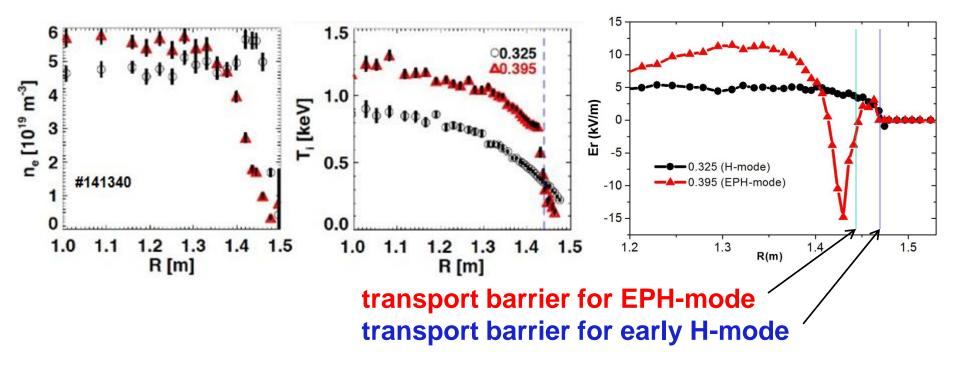
► location of EPH-mode transport barrier is close to  $\nabla^2 E \rightarrow 0$  area
