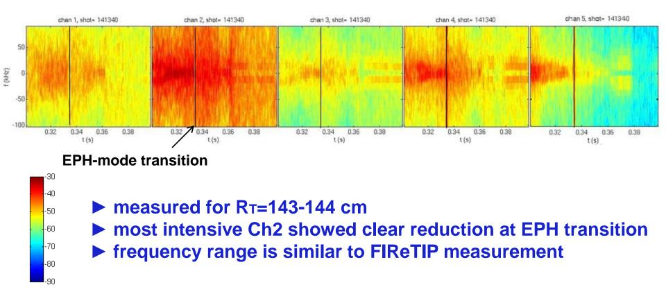
both FIReTIP and High-k showed fluctuation reduction on EPHmode transition at few cm inner location than normal H-mode transport barrier
