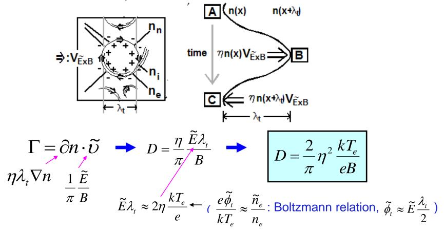
• turbulence induced ion and electron diffusion :  $\eta \lambda_t \nabla n$
