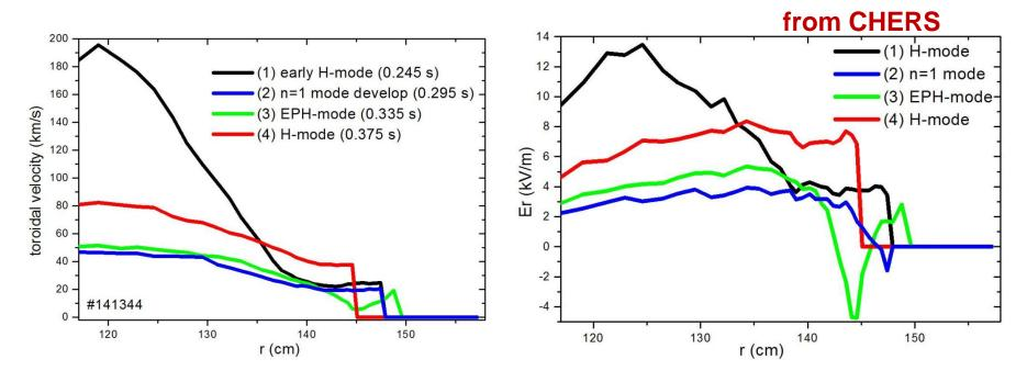
in stage (2), while n=1 mode develops, toroidal rotation decreases, and there is additional change in Er for boundary
