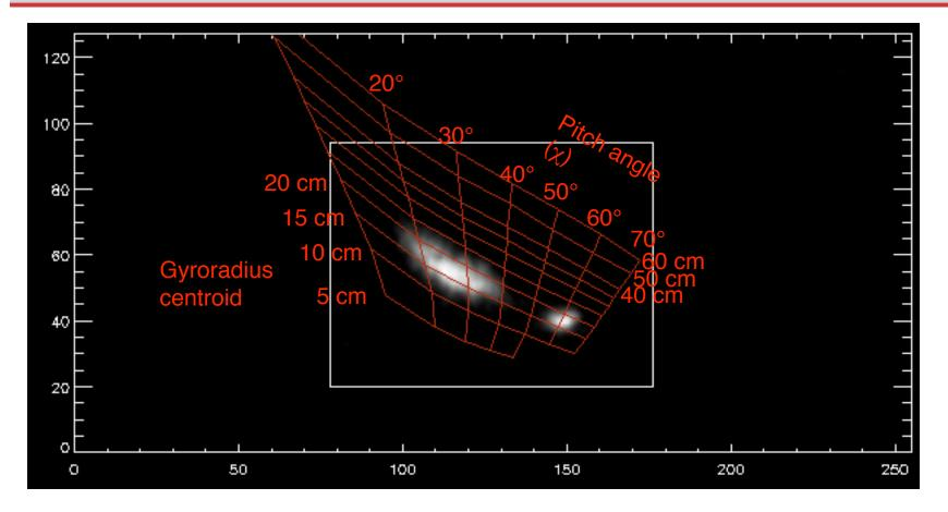
Rapid appearance of wide pitch angle spot (18°–40°) in 33 μs (≤10 toroidal transits) indicates transport of fast ions is very strong during avalanche
