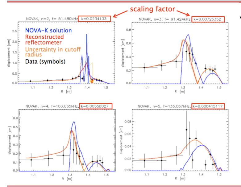
**Displace**ment can be matched, giving absolute amplitudes of various n modes for input into orbit following code
