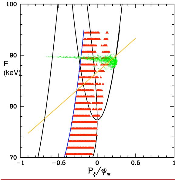
• Apparent good surfaces around  $P_{\zeta}=0 \& E> 85 \text{ keV}$ may prevent some of deposited population from reaching loss boundary
