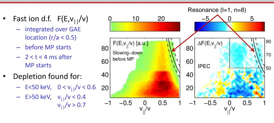
• GAE Doppler-shifted cyclotron resonances on the flank of the distribution function
