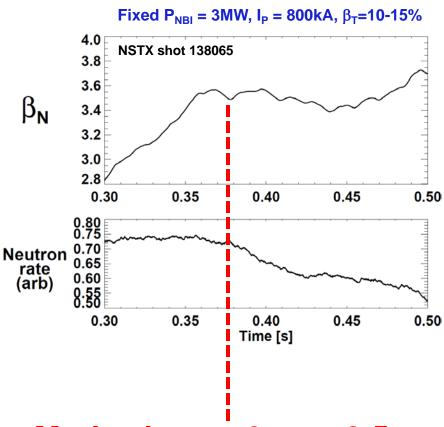
Mode clamps  $\beta_N$  to ~3.5, reduces neutron rate ~20%
