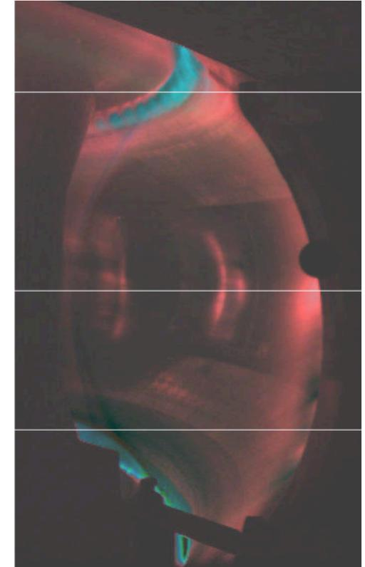
Shot 55851:  $P_{RF} = 2\text{MW}$ ,  $I_p = 400\text{kA}$ ,  $B_T = 2.45\text{ T}$  at  $R = 1.7\text{ m}$
