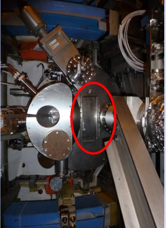
A 33 cm tall window at port L allows for  $k_{\theta}$  up to 40 cm<sup>-1</sup>.
