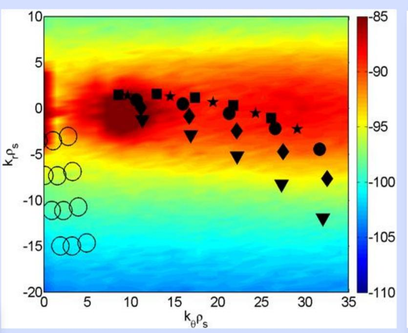
Computer simulation of ETG modes in NSTX-U. Peak modes are expected near  $k_{\theta} = 10 \text{ cm}^{-1}$  and  $k_r =$ 0 cm<sup>-1</sup>. Black symbols show possible coverage from the High-k Scattering System. The open circles show coverage from the previous High-k Scattering system.
