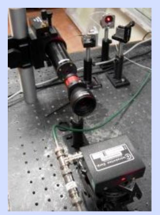
A 633 nm heterodyne interferometer is being utilized to detect changes in path length of the FIR lasers due to vibrations in the front-end optics and the internally-mounted retroreflector in real-time. The majority of the system consists of fiber optics for low-loss transport of the beam.
