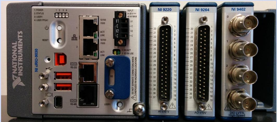
An FPGA will analyze and correct the FIReTIP signal for the effects of vibrations using input from the HeNe interferometer in real-time, allowing FIReTIP to be used for density feedback control.
