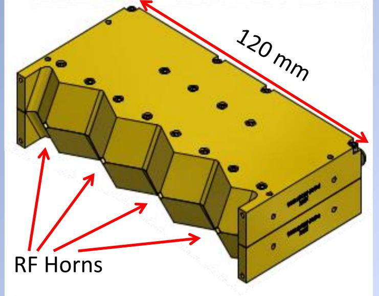
4x1 subharmonic, 693 GHz, mixer array from Virginia Diodes Inc. This modular design allows multiple arrays to be stacked for increased poloidal and radial coverage. Future developments will include an 8x2 array.
