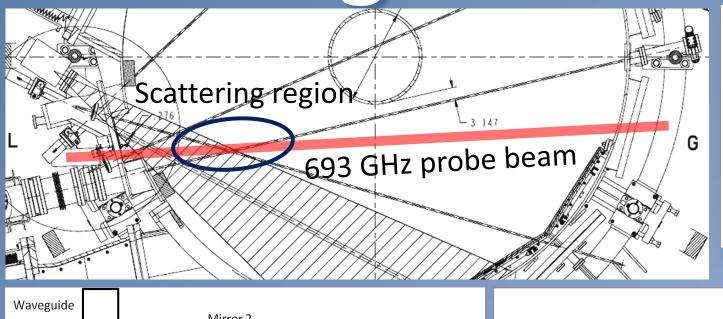
A series of mirrors and HDPE lenses will direct the 693 GHz probe beam from port G to port L.
