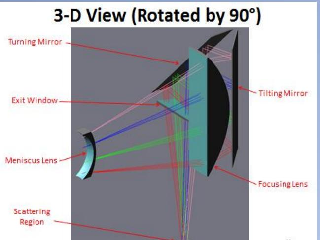
A system of remote control mirrors and HDPE lenses can target various locations in the scattering region. A meniscus lens redirects various scattering angles into parallel rays before being focused into the mixer input horns.
