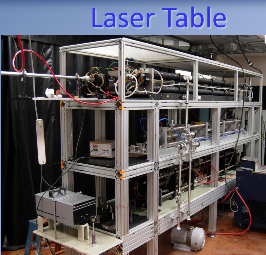
3 level laser table housing 6 lasers for High-k Scattering  $(1 \text{ CO}_2 \text{ pump}, 1 \text{ formic acid FIR})$  and FIRETIP  $(1 \text{ CO}_2)$ pump, 2 methanol FIR, 1 Stark effect methanol FIR ).
