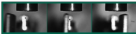
Horizontal injection of a 700 micron carbon microsphere. Exposure time is 50 microseconds and interframe time is 200 microseconds. Motion blur of the rightmost granule gives an estimated velocity of 45 m/sec.
