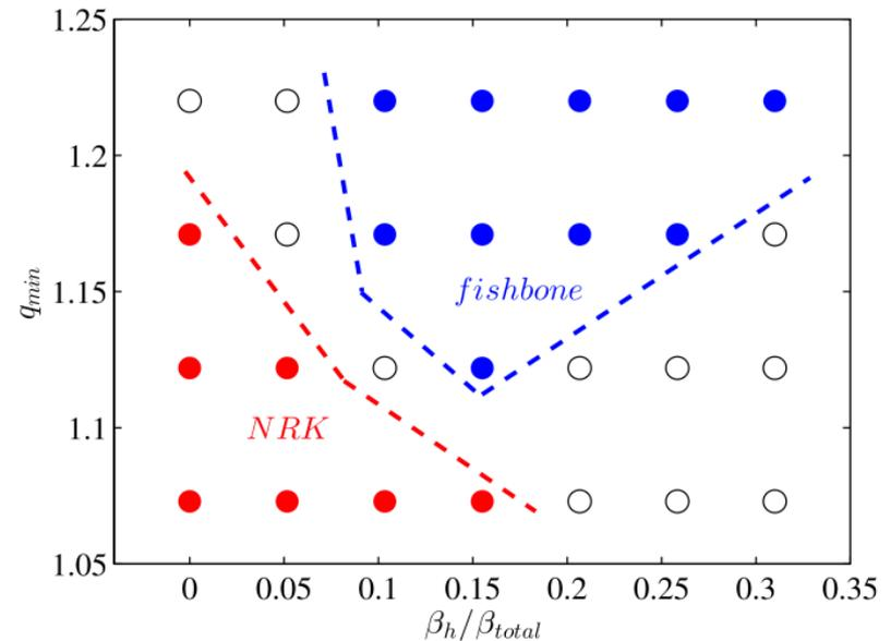
NRK/fishbone stability diagram from M3D-K simulations
