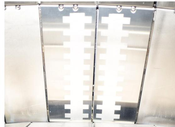
Sand blasted W tiles in ASDEX-U to increase emissivity
