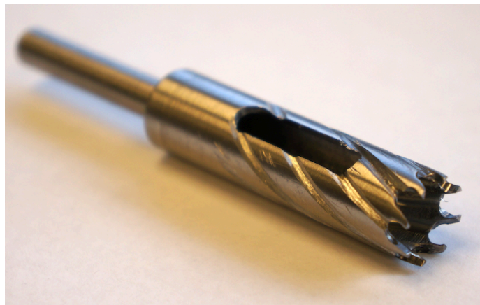
Precision, custom-made 3/8" i.d. core drill'
