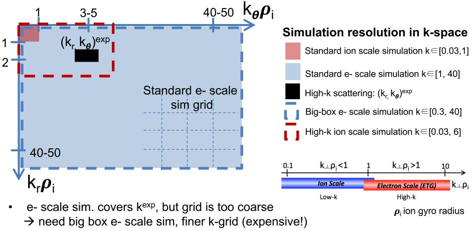
Ion scale sim. has good grid space, but does not cover k<sup>exp</sup>
