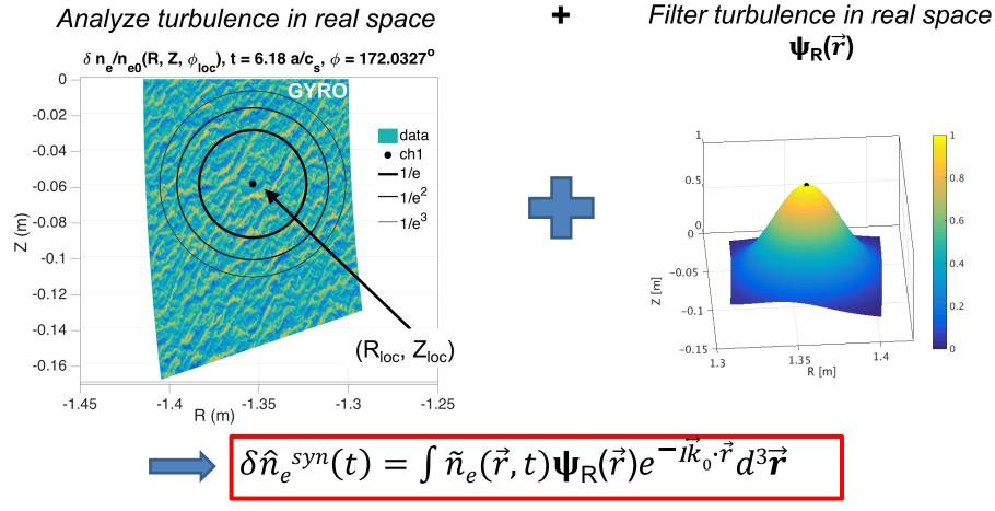
Obtain a time series of turbulent density fluctuations  $\delta \hat{n}_e^{syn}(t)$
