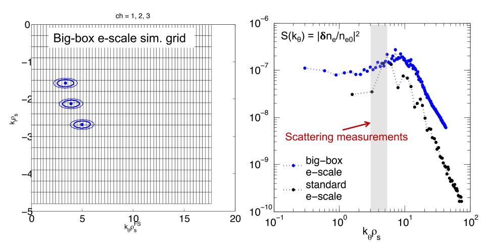
Big-box simulation spectra show well resolved (k<sub>R</sub>,k<sub>Z</sub>)<sup>exp</sup> and electron scale spectrum.
