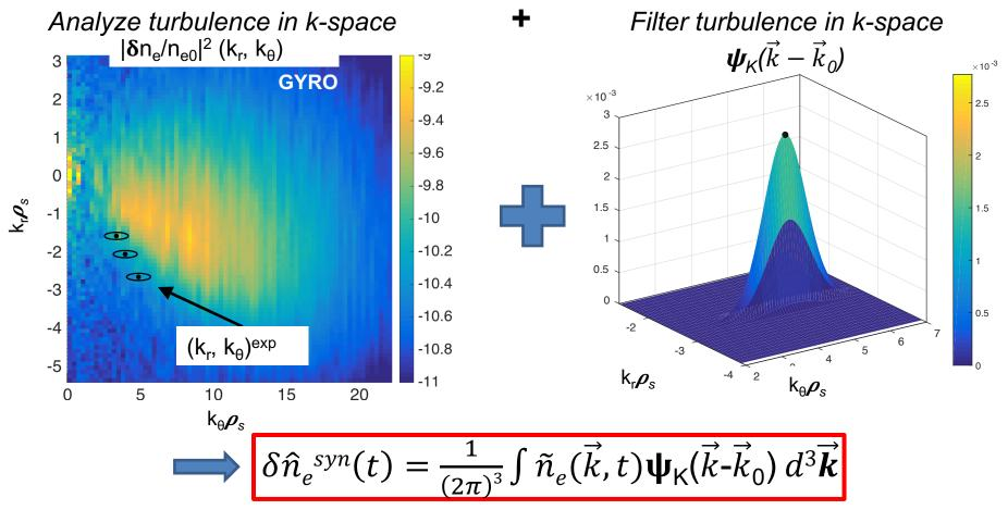
Obtain a time series of turbulent density fluctuations  $\delta \hat{n}_e^{syn}(t)$
