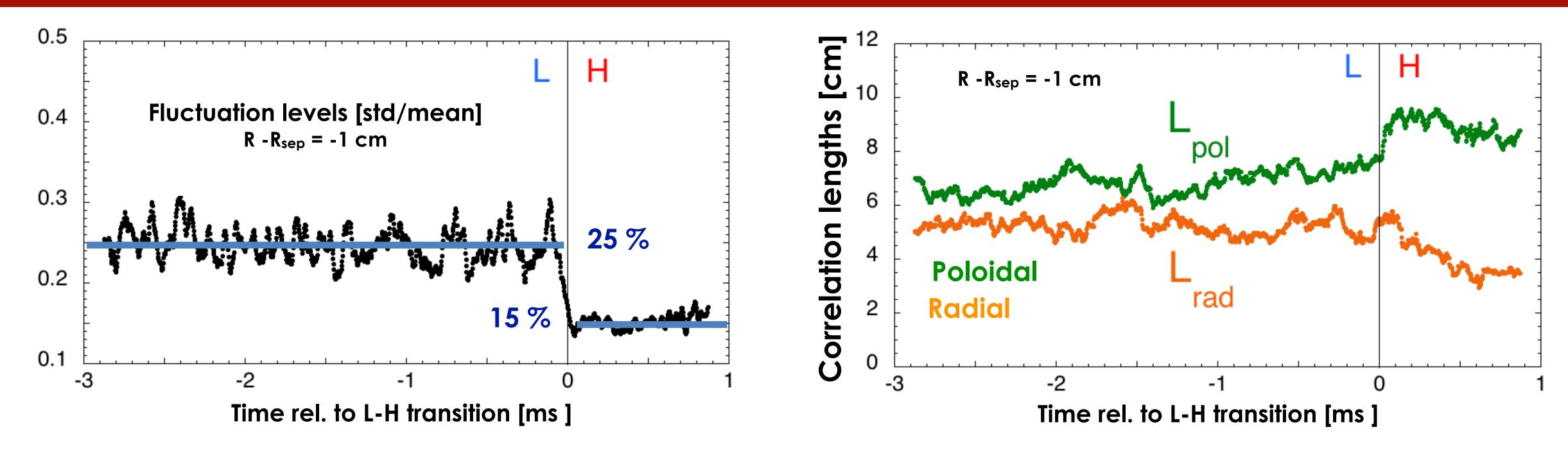
All turbulence quantities (averaged over 17 discharges) nearly constant at all radii up to 3 cm inside the separatrix during 3 msec before transition
