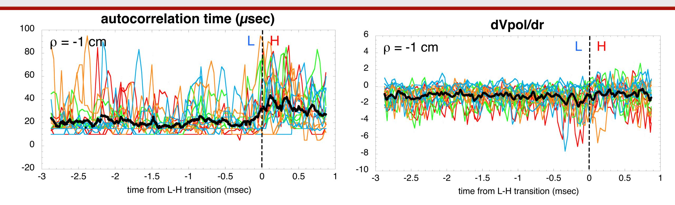
Average autocorrelation time =22  $\mu$ sec in L and 34  $\mu$ sec in H-mode Average  $dV_{pol}/dr = -1.1$  km/s/cm in L and -0.85 km/s/cm in H-mode
