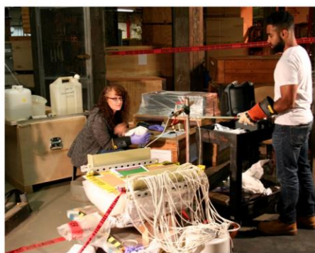
Technicians preparing for electrical testing of one of the sectioned PF1 prototype coils
