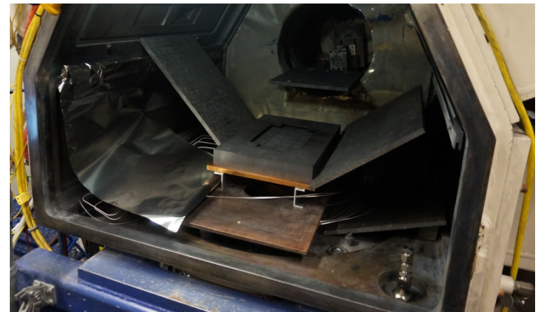
Castellated target installed in EB Facility
