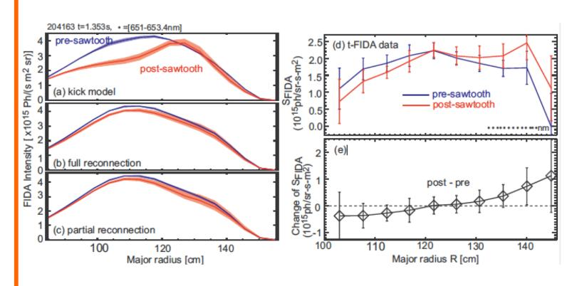
The kick model reproduces the observed asymmetry in the FIDA diagnostics, with a drop inside the inversion radius.
